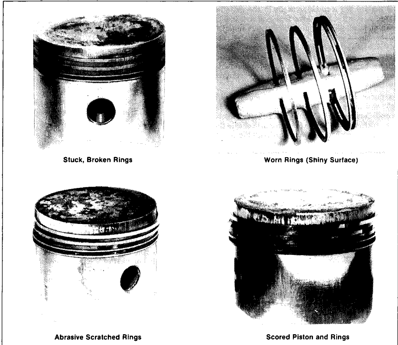
Figure 7-10. Common Sources Of Piston And Ring Damage
