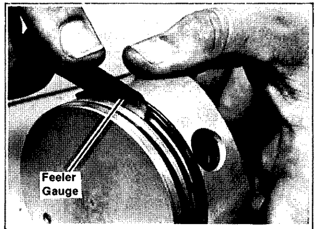
Figure 7-12. Checking Piston - Ring Side Clearance
