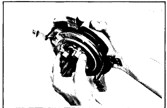
Figure 7-14. Removing Pulley From Housing.
