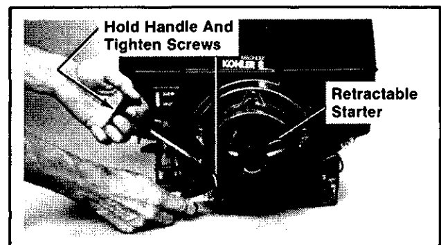
Figure 12A-38. Installing Retractable Starter.
