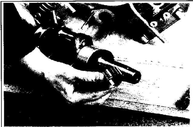
Figure 9-55. Belt Drive Sprocket Removed.
