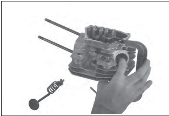
Figure 11-64. Installing Valves Using Valve Spring Compressor.
