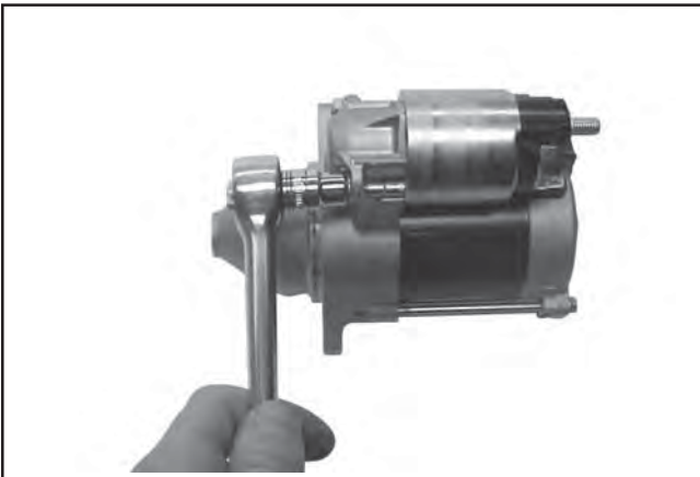
Figure 8-69. Installing Thru Bolts.
