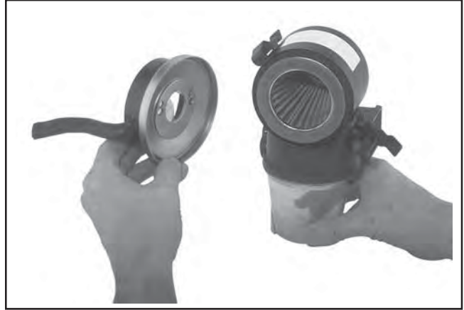
Figure 4-11. Installing Heavy-Duty Cover/Housing.
