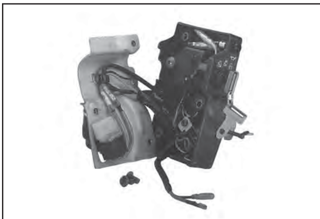
Figure 9-33. Control Panel and R.H. Tank Bracket.
