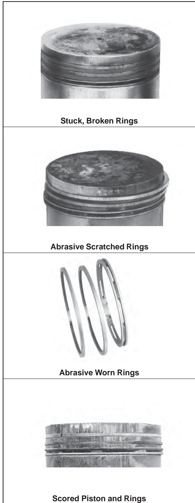
Figure 10-13. Common Types of Piston and Ring Damage.
