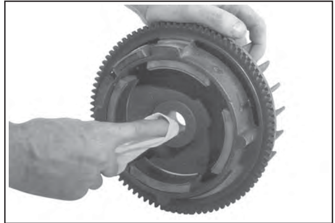
Figure 11-58. Clean and Dry Flywheel Hub.
