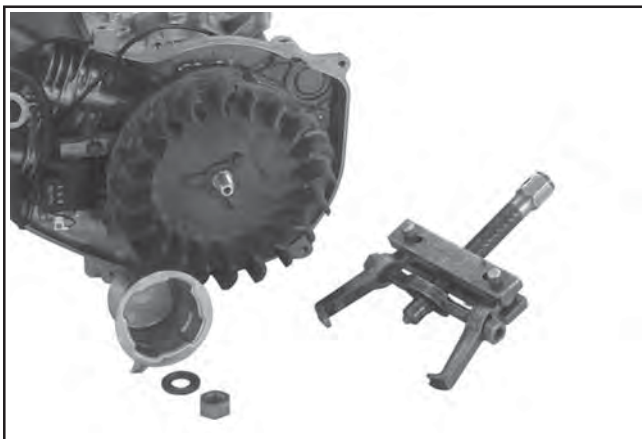
Figure 9-50. Use External Type Puller to Remove Flywheel on CS4, CS6.
