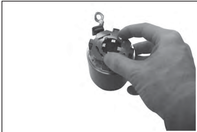
Figure 8-65. Holding Insulator in Place.
