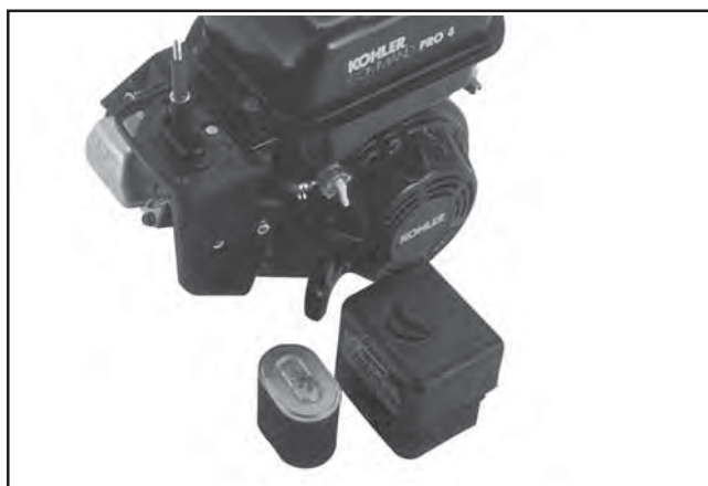
Figure 9-5. CS4, CS6 Air Cleaner Base.
