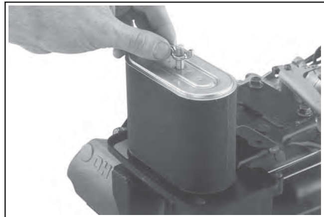
Figure 11-107. Installing Air Filter Element, Precleaner, and Wing Nut.
